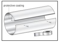
to ensure a good bond. Secure tube using the (2)  $\frac{1}{4}$  sheet metal screws (I) provided. Then place foil tape (F) over the entire seam to strengthen seal. When joining two pipe sections together; place the crimped end into the next section of pipe. Secure with a  $\frac{1}{2}$  sheet metal screws provided and seal joints with foil tape.
