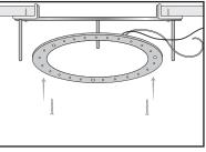
Note: The holes on the LED Ring will not line up with the holes on the Ceiling Ring. You must drill through the ceiling ring.
