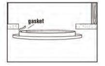
**STEP 5** Place the Ceiling Ring inside of the Anchor Ring. Line the countersunk screw holes on the Ceiling Ring with the larger holes on the Anchor Ring. Place the Ceiling Ring/Anchor Ring assembly in the hole cut in Step 2. Secure the assembly to the ceiling by inserting a 1½" Phillips
