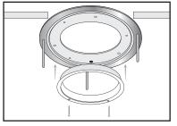
Screw (L) into one of the three countersunk holes and screw it through the drywall into one of the provided Speed Nuts (J). Repeat this process for the other two screws.
