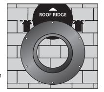
**STEP 12** Using a utility knife, cut a four-inch slit through the shingles and tar paper at the 3 o'clock and 9 o'clock positions of the hole cut in step 11. This allows for the footprint of the flashing to be inserted under the shingles.
