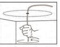
as close to the desired installation area as possible. Mark the center of the Ceiling Ring, drill a hole and insert piece of wire bent at a 90-degree angle. Rotate the wire around 360 degrees. While rotating, feel for resistance that could indicate wire runs or other obstructions.
