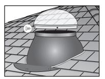
**STEP 22** Replace the Decorative Diffuser Cover and Silver Trim by placing the Silver Trim in the groove at the bottom of the Decorative Diffuser Cover. Align the 3 holes in the Silver Trim up with the prongs on the Anchor Ring, and use the screw covers to secure it.
