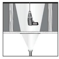
With a drill bit and appropriate extension rods, drill a pilot hole in the marked location on the bottom side of the roof.
