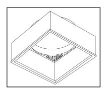
**STEP 15** Replace the Diffuser on the Transition Box by placing the flat tabs inside the frame first and then pushing the diffuser in place.
