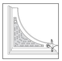
STEP 10 One by one, place and secure the LED Quadrants into the each corner of the Transition Box by drilling the screws into the Transition Box, so that the LEDs face downward towards the room and quadrants are flush against the transition box.
