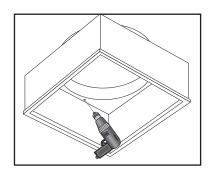
STEP 17 From the roof, slide the light pipe assembly with the crimped edge down into the transition box collar. Secure the light pipe to the flashing with the (4) Phillips flat head 1 ½" screws (D) provided through the (4) pre-drilled holes on the flashing
