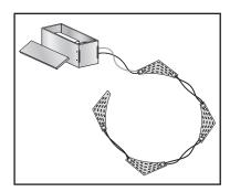
STEP 14 Secure the LED Driver Enclosure to the Transition Box by feeding the hollow, threaded bolt through the 1/4" hole cut in step and tightening one nut inside the Transition Box and one nut outside of the Transition Box.
