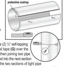
a good bond. Secure tube using the (2) ½" self-tapping screws **(H)** provided. Then place foil tape **(G)** over the entire seam to strengthen seal. When joining two pipe sections together, place crimped end into the next section of pipe. Secure the connection of the two sections of light pipe with (2) ½" self-tapping screws provided and seal joints with for
