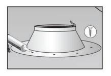
then next directly across from it at 6:00. The third screw should go at 9:00 and the next screw directly across at 3:00, etc. Caulk over the screw heads, since they will be exposed to the weather.
