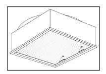
STEP 8 Peel the protective backing off the white nylon horsehair gasket (I) and apply gasket on the INSIDE COLLAR OF THE TRANSITION BOX (J) ½" down from top of the collar.
