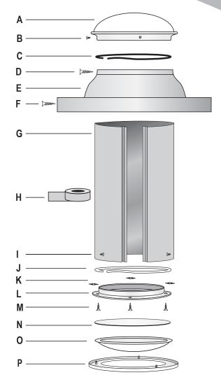
**IMPORTANT:** Prior to beginning installation, it is critical to plan the placement of the tubular skylight so that curb flashing and ceiling trim ring are aligned. Ensure that the curb is not installed over any framing trusses. DO NOT CUT ANY STRUCTURAL FRAMING.
